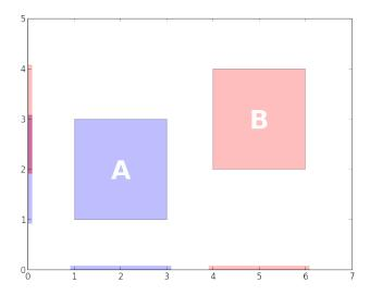
The full set of the RA relations is determined by *Allen's Interval Algebra* relations. Therefore, since there are 13 Allen's relations, RA defines 169 possible relations over the xy segments of two rectangles.
