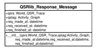
The information returned by QSRlib is an object of the class QSRlib\_Request\_Message, which mainly consists of the computed QSRs in the *qsrs* member and is a *World\_QSR\_Trace* object. If requested, a graph representation of QSRs, which contains additional temporal information about them is also returned in the *qstag* member.
